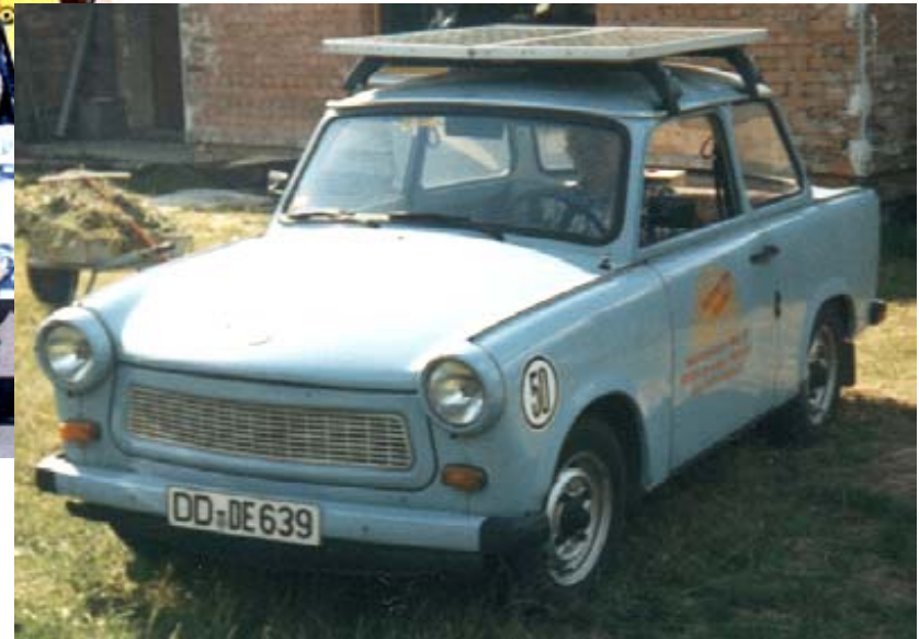
Trabi, Dresden, with 200 Watt photovoltaik modules
