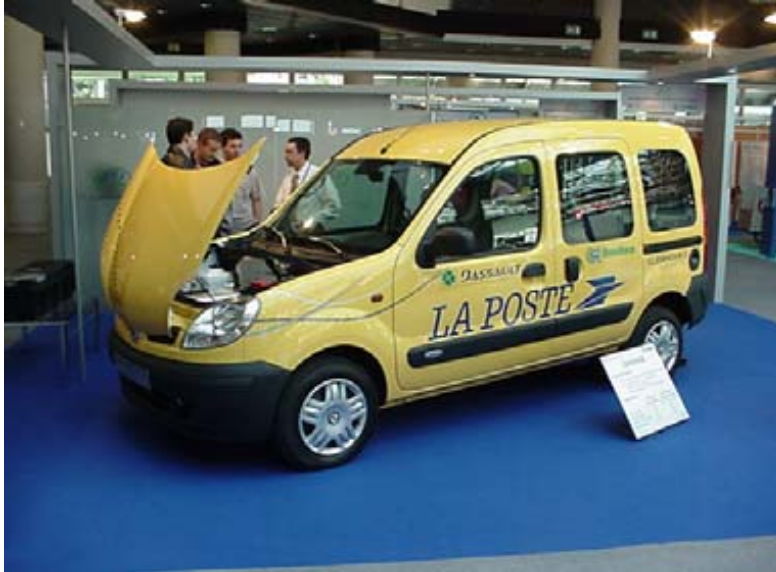
Left: Kangoo electric RE, hybrid car with range extender and SAFT lithium batteries, special project for „La Poste“, France, made by SVE - Société de Véhicules Electriques
