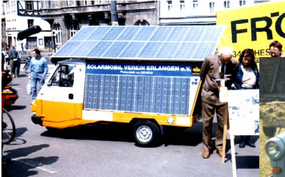
First German Solar Vehicle for everyday use Solarmobil Verein Erlangen e.V. 600 Watt solar generator
