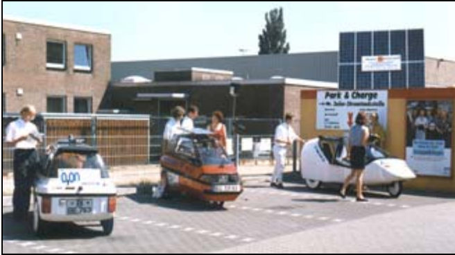
City-El and TWIKE at a Park & Charge solar charging station
