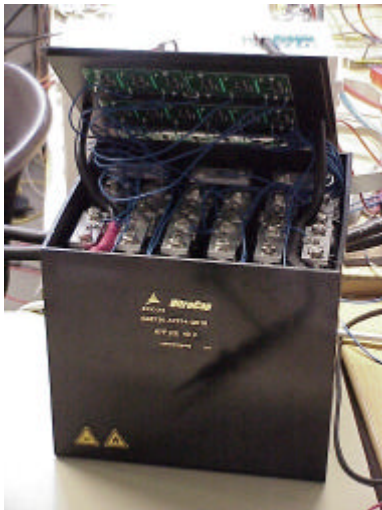
Fig 1: Ultracap module with charge balancing unit – Bench test indicating all cell voltages within their limits
